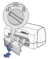
2 Press the button on each side of the Automatic Two-Sided Printing Module, and insert the module into the back of the printer.
